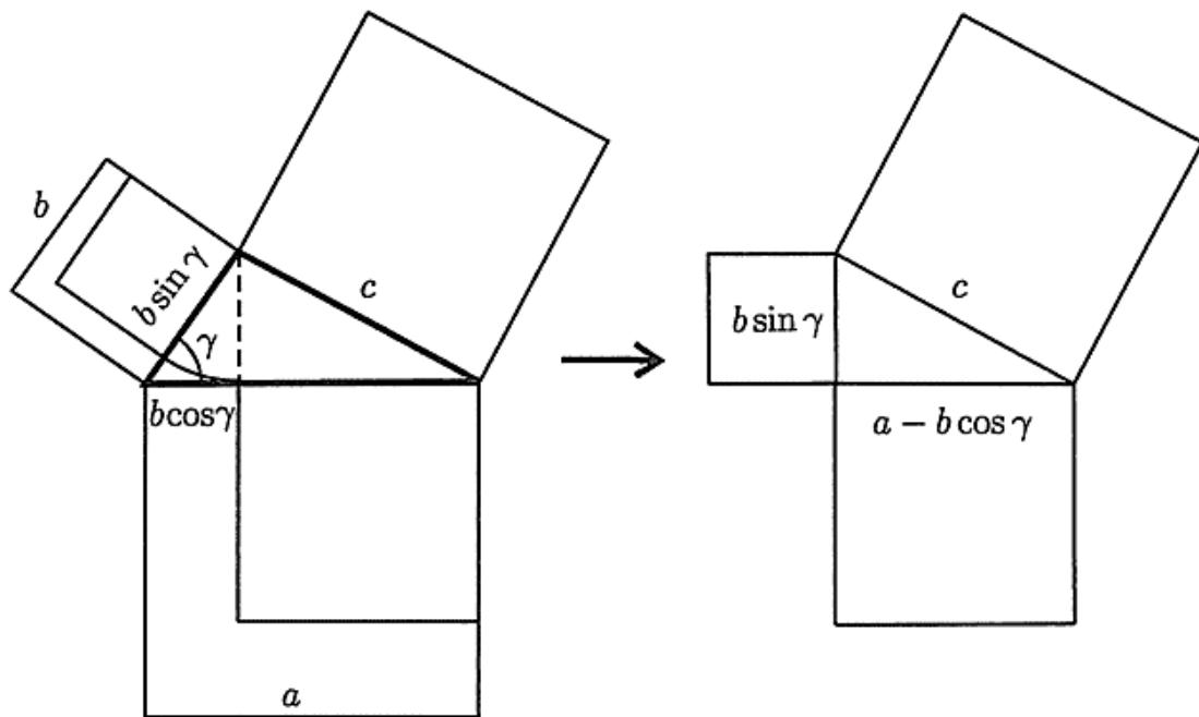
$$\begin{aligned} c^2 &= (b \sin \gamma)^2 + (a - b \cos \gamma)^2 = b^2 \sin^2 \gamma + a^2 - 2ab \cos \gamma + b^2 \cos^2 \gamma \\ &= a^2 + b^2 - 2ab \cos \gamma \end{aligned}$$
